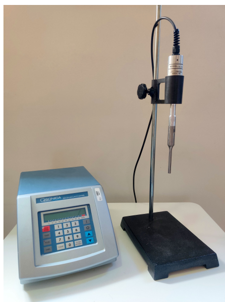
Figure 3.3: Qsonica Q125 Sonicator ultrasonic processor with standard probe.
