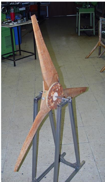
Figure 2.28: Stand used to perform the rotor's calibration [15].
