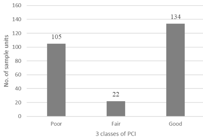
Figure 3. PCI distribution by 3 classes: Poor (0–55), Fair (56–70), and Good (71–100).
