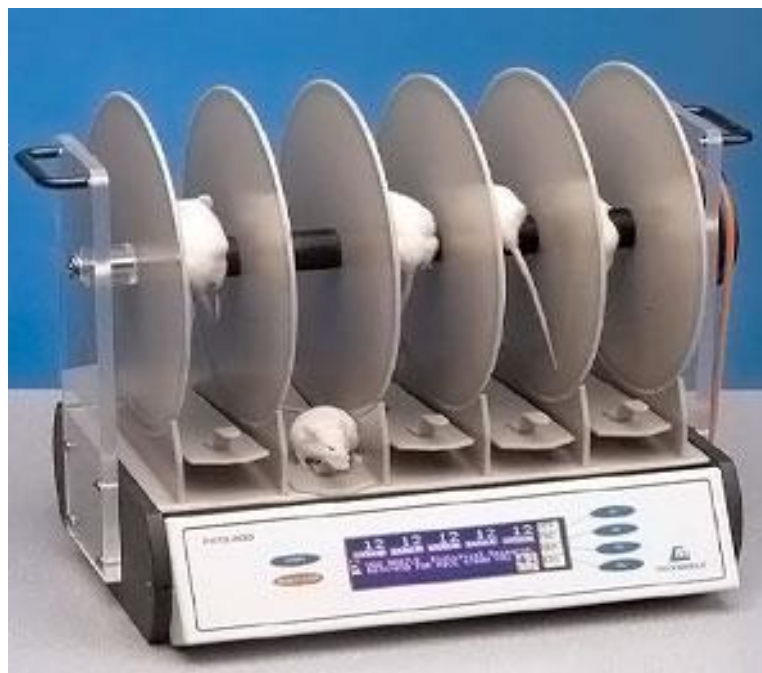
Figure 9. The rotorod treadmill measures motor coordination in rodents. In each lane a rodent is placed. The rodents are exposed to drugs or vehicle. Notice the platform beneath the rotating cylinder. When rodents fall off the cylinder into the platform the timer stops. The quicker the rodents fall the lower their motor coordination.
