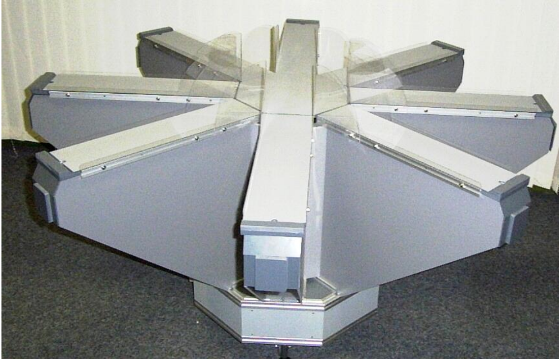
Figure 10. The radial arm maze. Used to assess working and reference memory in rats and mice. When investigating working memory, all arms are usually provided with a reward and the animal should visit each arm only once. When used for assessing reference memory, only some of the arms contain a reward and the animal should only visit those baited arms. Visits to an arm more than once or visits to non-baited arms count as working memory errors or reference memory errors, respectively.
