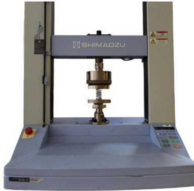
Figure 81 Experimental determination of spring k using the SHIMADZU® AGS-X.
