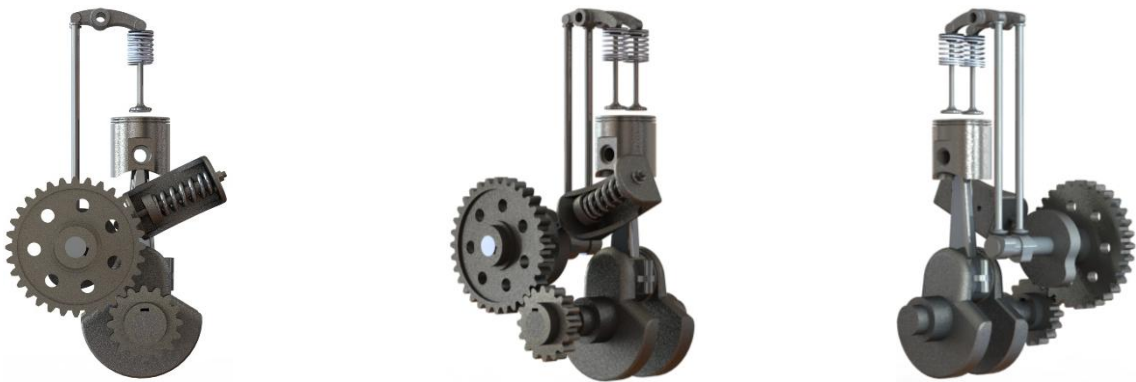
Figure 79 CAD model of the proposed balancing cam mechanism, designed to produce a counteracting torque at various crankshaft angles, with direct implementation in the camshaft.
