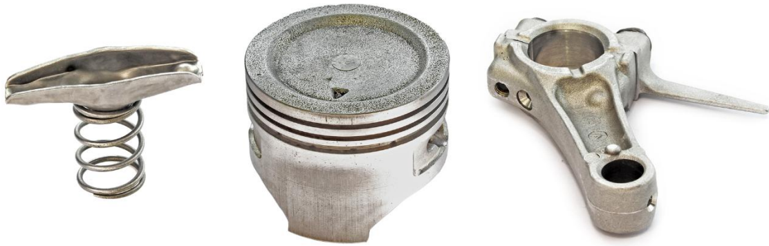
Figure 45 Rocker arm from valve mechanism, piston and connecting rod from Honda® GX 120 engine.
