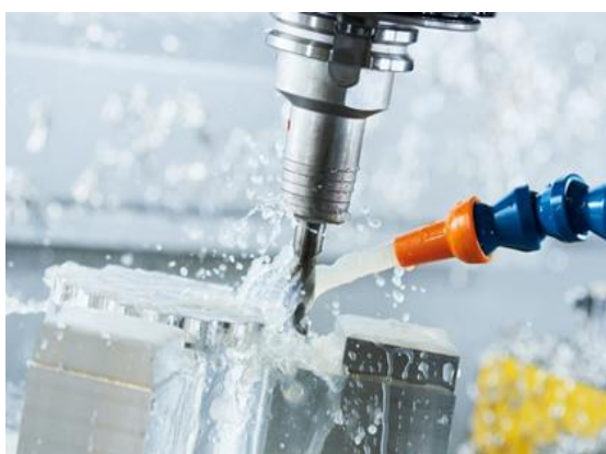
Figura 26 - Refrigeração externa (Ridgeback Engineering Supplies, 2021).
