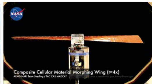
Figure 2.4: Ultra-light composite cellular material morphing wing prototype [4].
