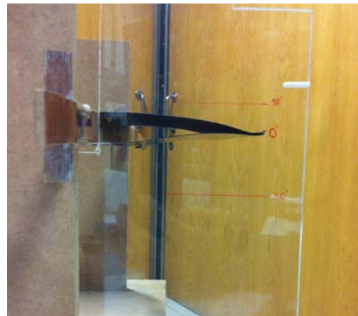
(b) Flap's shape with no applied loading.
