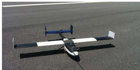
Figure 1.3: Olharapo II fitted with the VSW concept from CHANGE technology proceedings.
