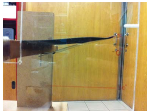
(d) Flap's shape change - 10^\circ up.
