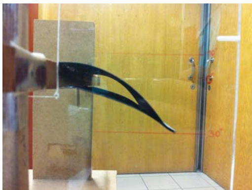
(c) Flap's shape change - 30^\circ down.
