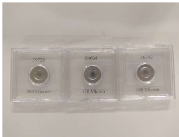
Figure 2.10: Stainless-steel high precision optical pinholes with an inner diameter of 200\ \mu\text{m} , 150\ \mu\text{m} , and 100\ \mu\text{m} .
