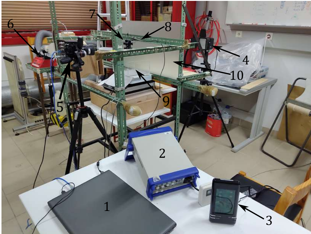
Figure 2.12: Experimental Arrangement: 1) Computer; 2) Signal generator; 3) Temperature sensor; 4) Halogen lighting unit; 5) High-speed digital camera; 6) Syringe pump; 7) Droplet generator; 8) Picoscope tip; 9) Liquid reservoir; 10) Diffuse glass.
