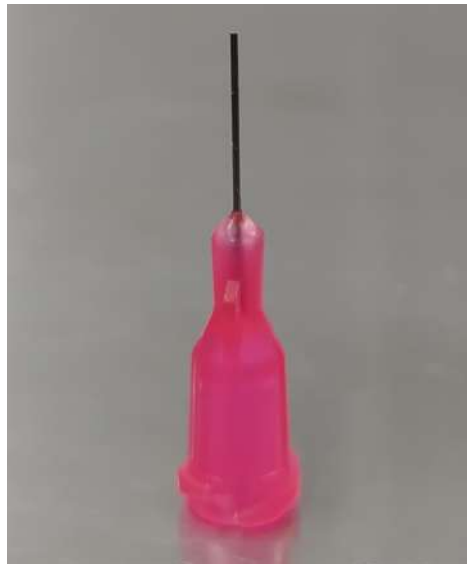
Figure 2.18: Stainless steel dispensing needle with an outer diameter of D_{out} = 510\ \mu\text{m} .
