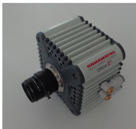
Figura 4.17: Câmara Digital CCD C10600-10B Orca-R2 com lente C-mount OPT-MHR31214MCN, de 12 mm.
