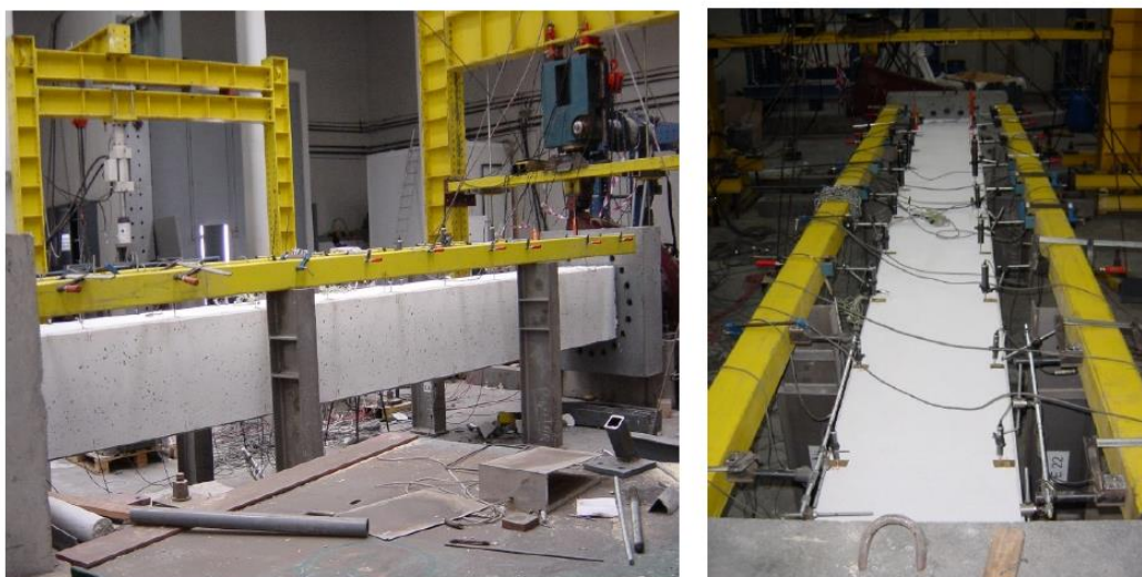
Figure 7. Beam specimen in test position.
