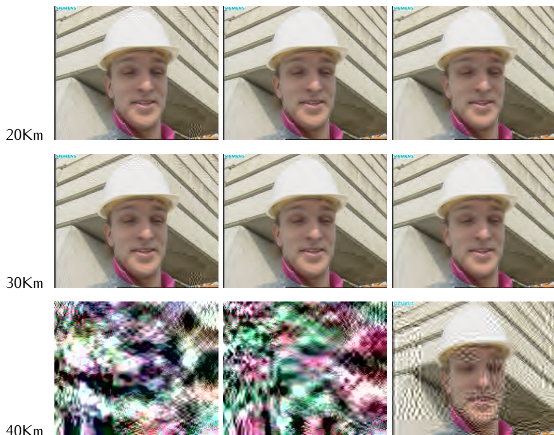
Figure 4.3: Simulation results for transmission over 20, 30 and 40 km with 0.0, 0.2 and 1.0 redundancy, respectively.
