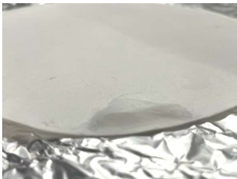
Figure 4. 7 - Emulsified cellulosic structure attached to the blotter to mimic a layered system that could be applied to the skin as a dermic system.
