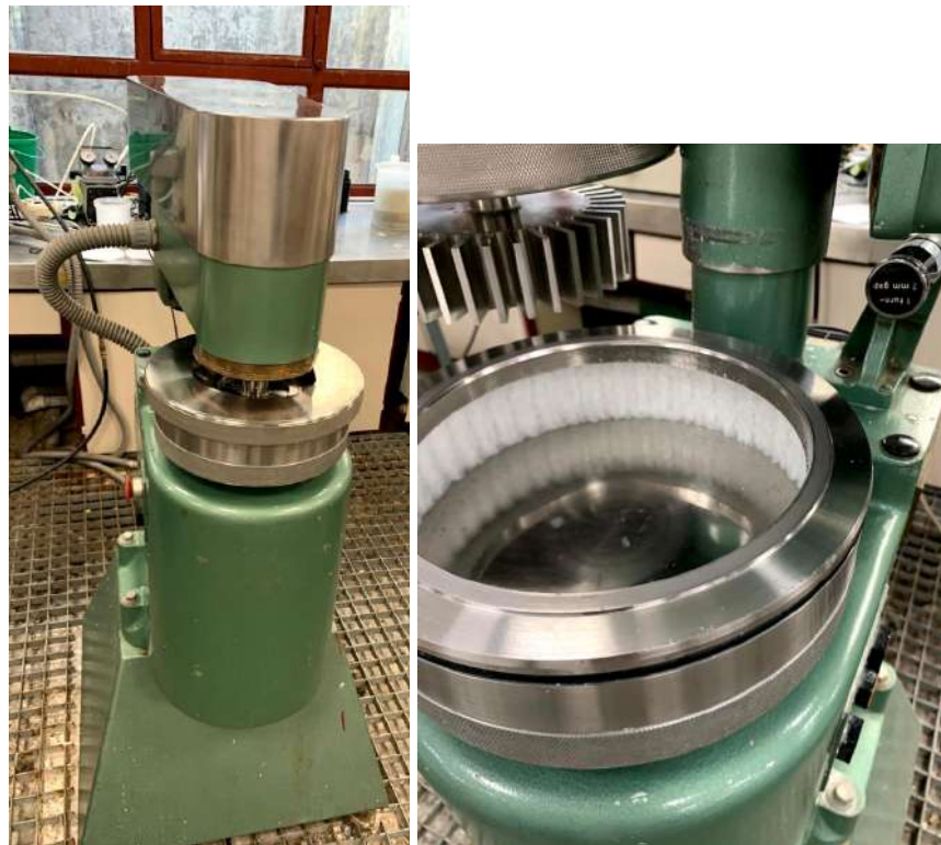
Figure 3. 1 - Representation of the PFI mill equipment, that was used to refine fiber, in which (a) overall representation of the equipment and (b) visualization of cellulosic fibers on the walls of the container that is placed on the bottom
