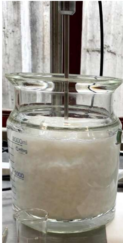
Figure 3. 2 - Representation of the reactor where it was made the enzymatical treatment of the cellulosic fibers
