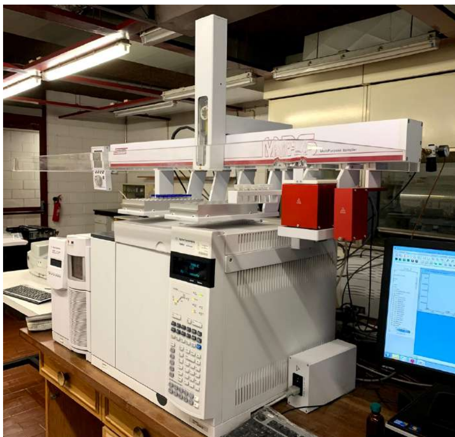
Figure 3. 4 – Agilent technologies 7890A GC A.01.13 with Agilent Technologies 5975 inert XL MSD with Triple-Axis Detector representation
