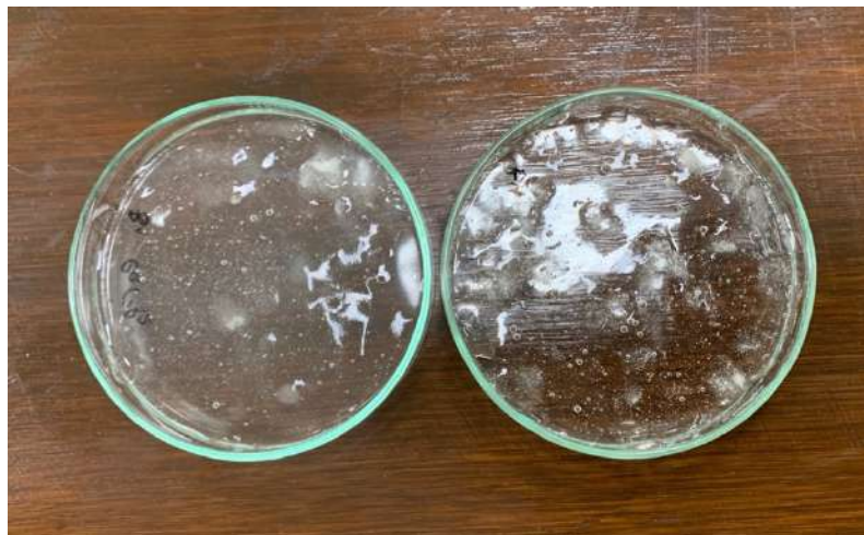
Figure 4.20 - Hydrogel made with 1600mg CMC + 400mg CaCl 2 (left) and hydrogel made with 1600mg CMC (right).
