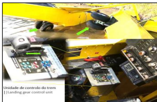
Figure 10 - Fireboss Landing Gear control panel [39].
