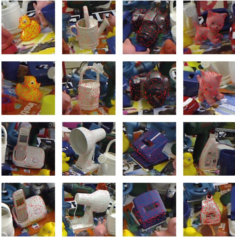
Figure 1.1: 6D Pose Estimation Example. The red dots represent the object keypoints of the estimated 6D pose projected onto the RGB image.
