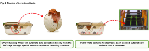
Fig. 2 The DVC® Running Wheel allows to automatically record data on the use of the Running Wheel by mice. This automatic data collection will provide not only information on the use of the Running Wheel but also the total distance covered. Fig. 3 Digital ventilated cage (DVC®) is a commercial system designed to collect information directly from the cage. The DVC® board is composed of 12 electrodes connected to an integrated circuit that continuously measures their electrical capacitance. The movements across the electrode array are detected and recorded as alterations in capacitance. By applying custom-designed algorithms to the collected data we can infer information regarding in-cage animal activity.
