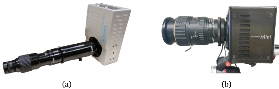
Figure 4.5: a) CR600x2 high-speed camera with a magnifying lens Zoom 6000®; b) Photron FASTCAM mini UX50 with 1.3 Megapixel.
