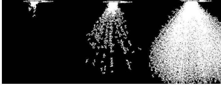
Figure 5.12: Visualization of the binarization of the spray using several frames.
