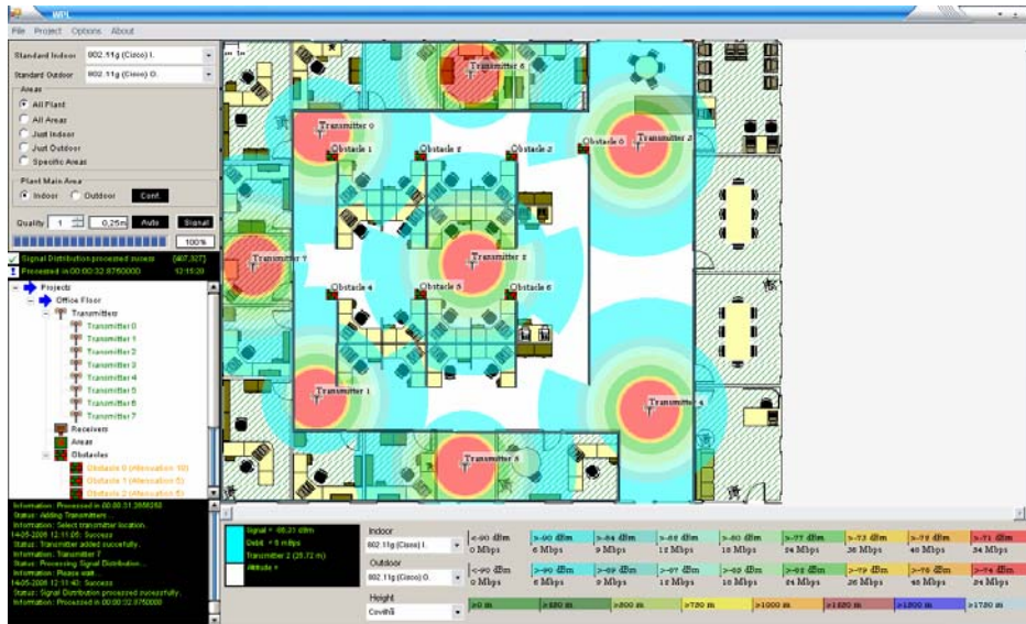
Fig. 3. WPT layout with indoor application.
