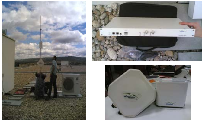
Fig. 5. IEEE 802.16-2004 PTM equipment operating at the 3.5 GHz (licensed) band.
