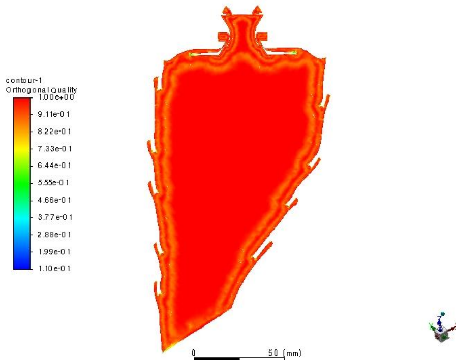
Figure A.E.1: Contours of orthogonal quality in the cells in the cut-view plane of the first swirler, obtained with ANSYS Fluent software.
