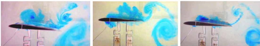
Figure 2.12: Wake structures under different kinematics (trapezoidal, sinusoidal, and triangular from left to right) [66].
