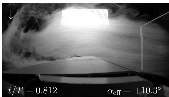
Figure 8.9: Flow visualization at Re = 1.0 \times 10^4 , h = 0.25 , k = 1.0 and A_\beta = 10^\circ at t/T = 0.812 .
