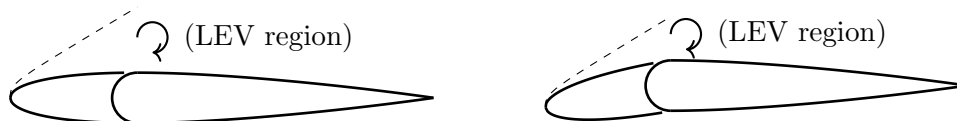
Figure 8.44: The growing mechanism of the leading-edge vortex. The shear layer is illustrated as the dashed line.
