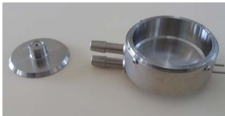
Figure 2.17: Cone and plate geometry.
