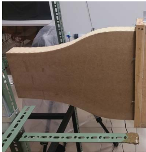
Figure 2.4: Wind tunnel contraction ( CR = 2 ).
