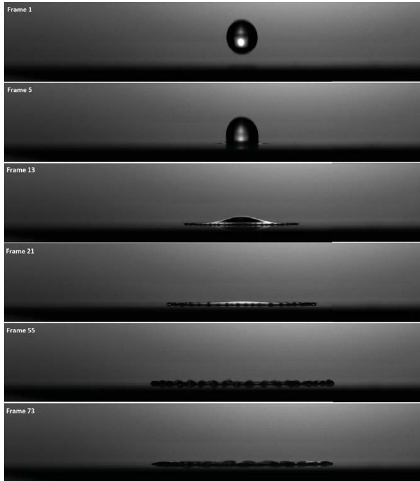
Figure 3.3: An H_2O droplet impinging onto an aluminum plate ( D_0 = 4.06mm ; Re = 15588 ; We = 828 ; La = 293454 ).
