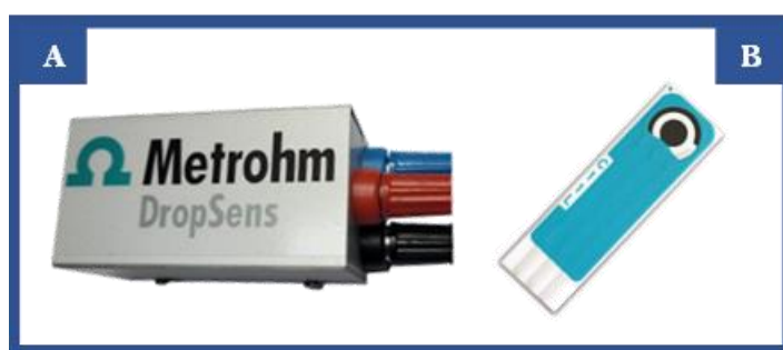
Figura 2.2: (A) Caixa conectora DropSens (DRP-DSC). (B) Chips C-SPE DropSens (DRP-C110).
