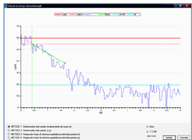
Fig. 9. Graphical representation of the sound pressure level decay experimentally measured.
