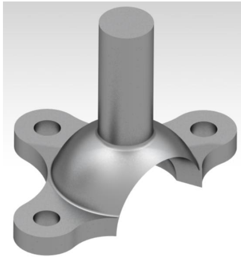
Figure 4.4 - Socket and connecting rod ball joint cap with crosshead engagement pin in CATIA V5
