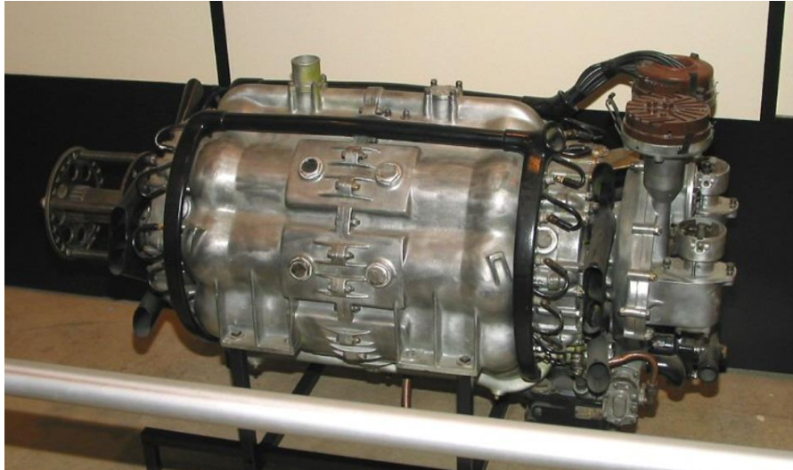
Figure 2.10 - Almen A-4 axial opposed-piston engine [14]
