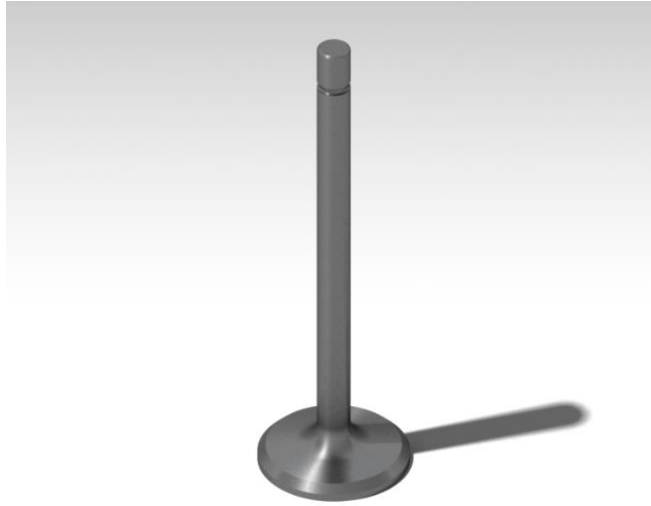
Figure 4.29 - Exhaust valve “Ferrea F6312 6000 Series” in CATIA V5
