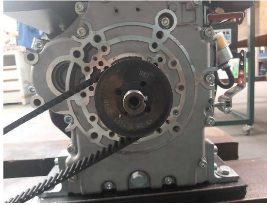
Figure 3.26. Pulley and taper lock bush in engine shaft.
