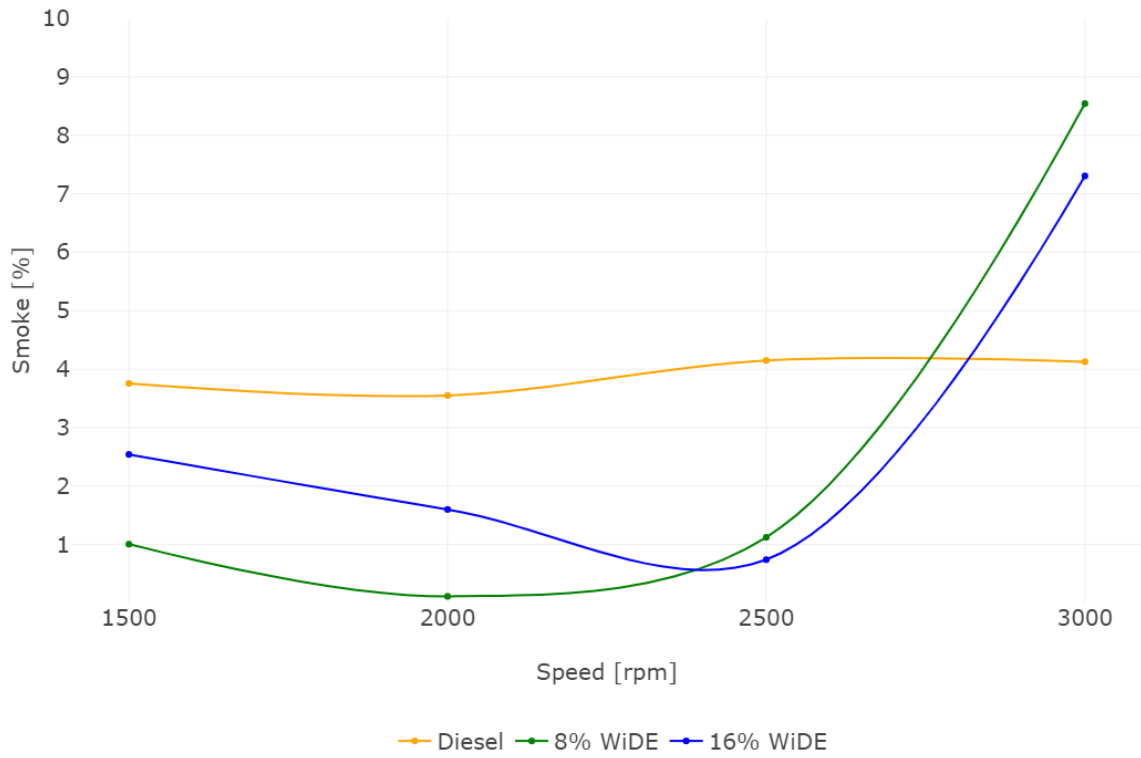
Figure 4.76. Smoke emissions at 50W load.
