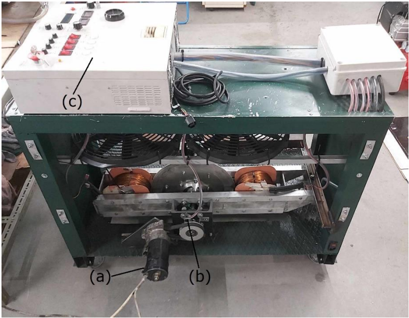
Figure 3.12. Engine test-bench (rear-view) – (a) starter motor, (b) hall sensor, and (c) dynamometer controller.
