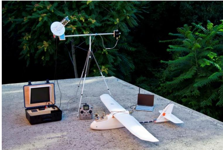
Figure 4- Complete UAV System
