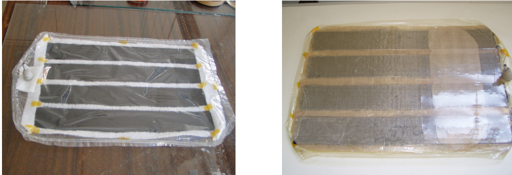
Figure 3.4: Specimens before and after the curing process
