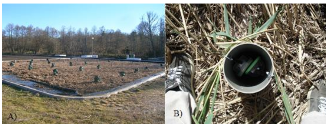
Figure 4.26 - A) Network of measuring tubes with sensors. B) Sensors inserted into a tube.
