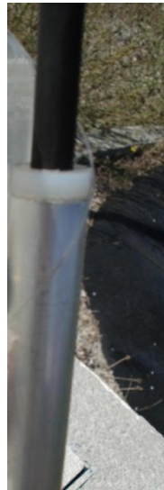
Figure 4.6 - Plastic cap placed on the top part of the sensor.
