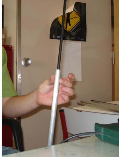
Figure 4.5 - Solid aluminium rod being inserted into hollow aluminium rod.
