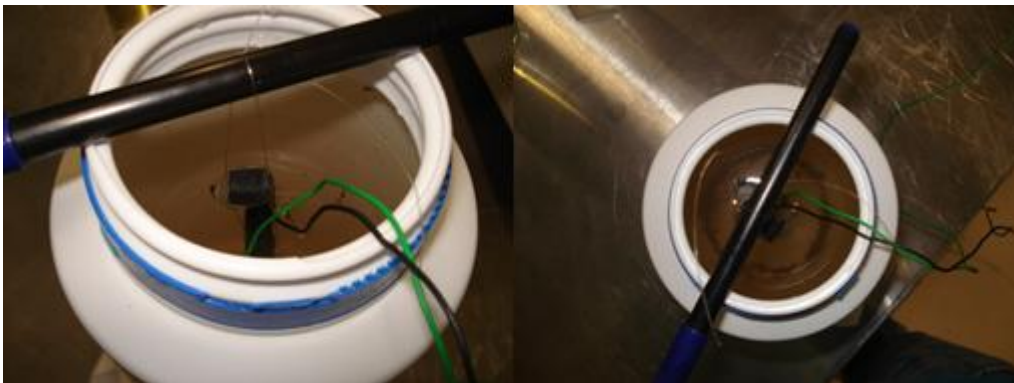
Figure 4.18 - Capacitance measurement with samples from HSSF-CW.
