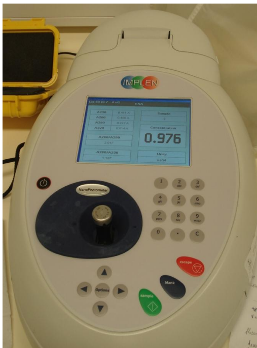
Figura 16 - NanoPhotometer (IMPLEN, Munich, Germany) usado para quantificar as amostras de RNA
