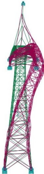
Figure 3.43 Global buckling shape of the bridge
