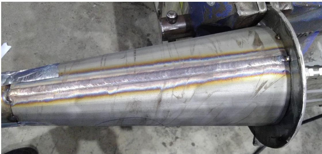
Figure 4.5- TIG Full Penetration Welding in the Combustion Chamber.
