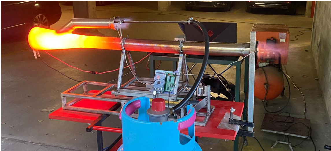
Figure 5.4-Pulsejet during a static test.
