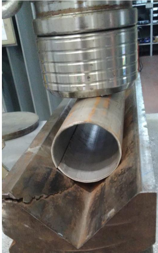
Figure 4.4-Press to give the final shape to the Combustion Chamber.
