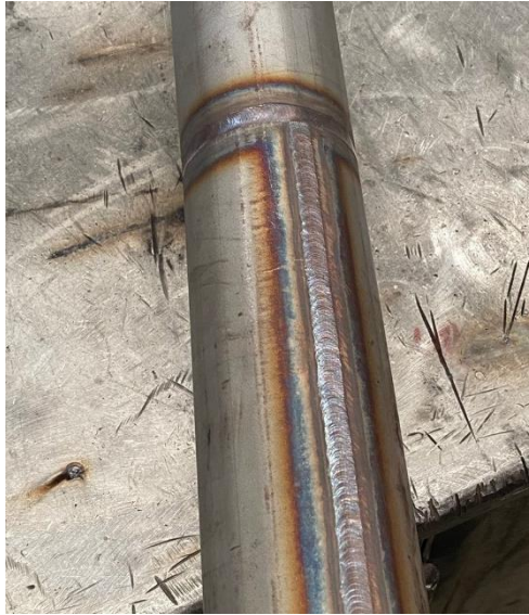
Figure 4.7- TIG Full Penetration Welding in the Exhaust.
