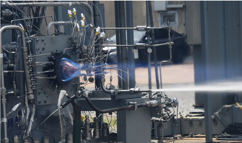
Figure 2.1: A prototype RDE under test at the Marshall Space Flight Centre. [8]
