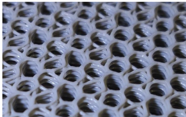
Figure 49 – Close up of the humidifier cells in which porosity and water accumulation is visible.
