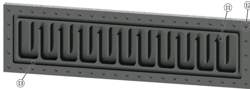
Figure 42 – Rendered view of the HX aluminium plate.
