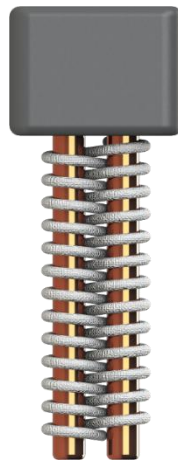
Figure 113 – Simplified representation of a two electrode FMRS.
