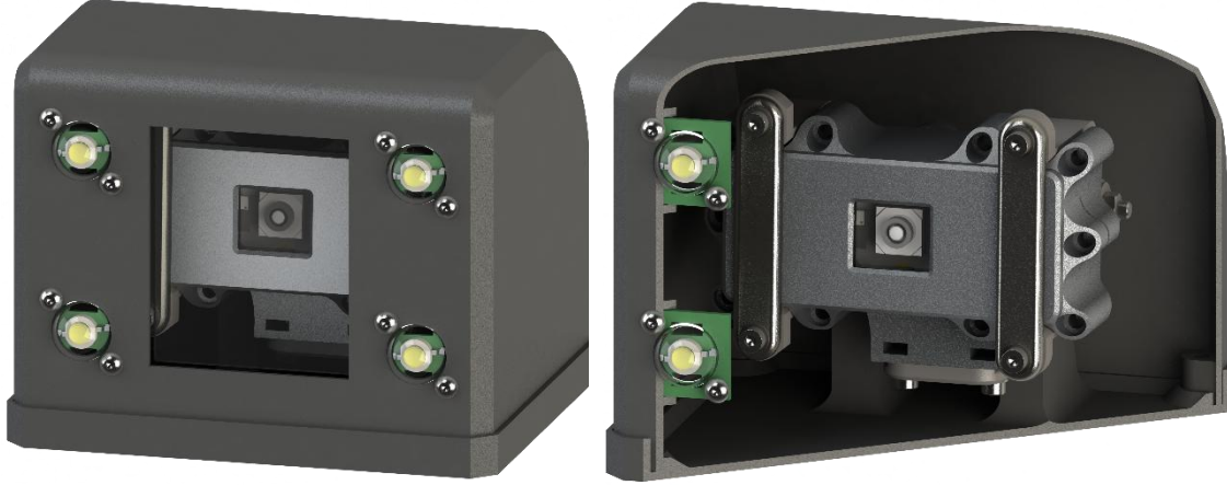
(a) (b) Figure 230 – Assembled CAD drawing of the whole system (a) and a cut view showing the inside the first enclosure (b).
