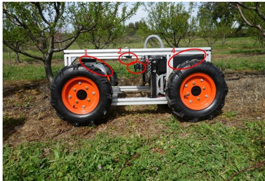
Figure 5. Robotic Rover for agricultural applications: (1) herbicide reservoir; (2) camera; (3) Cartesian robotic manipulator with spray nozzle; (4) control system.
