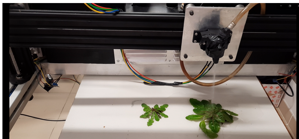
Figure 15. Result of real-time application: positioning of nozzle and spray atomization.
