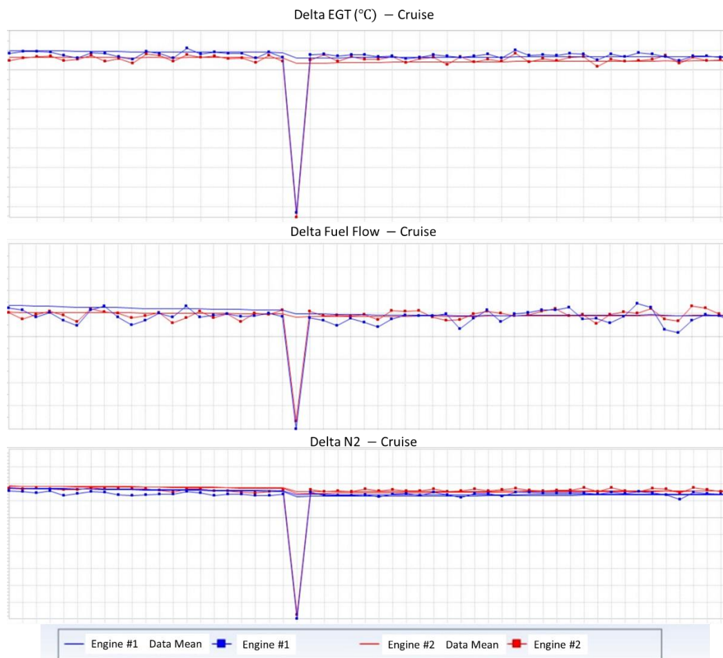
Figure 4.2 – Example of trend shifts on both aircraft engines due to aircraft total air temperature probe malfunction.
