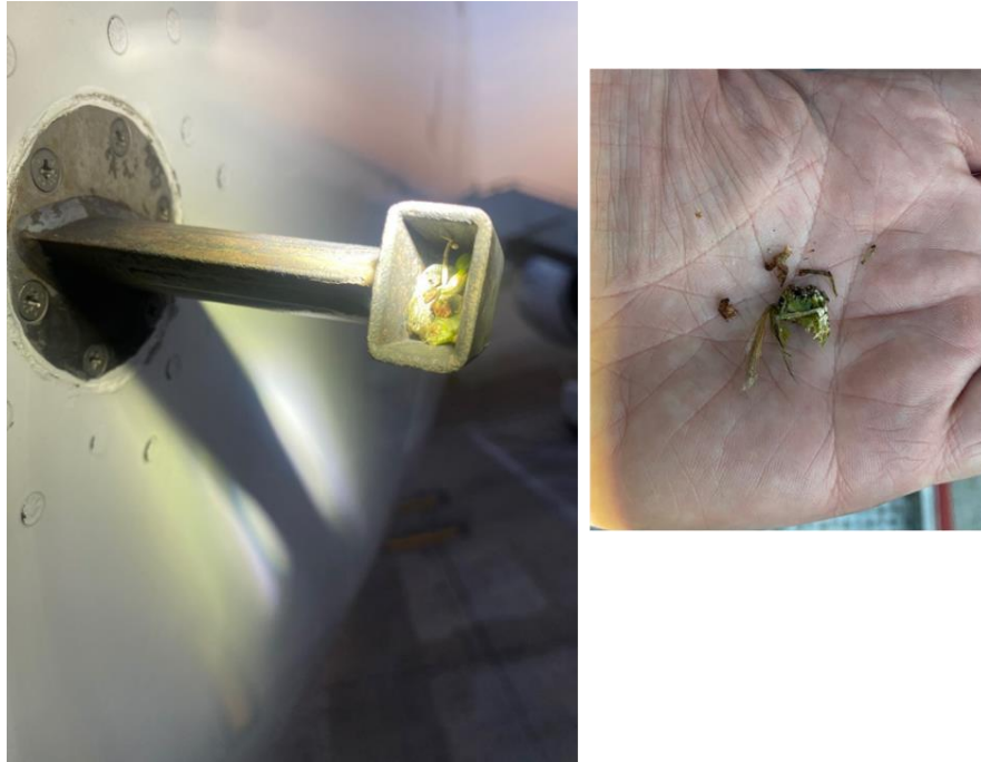
Figure 4.3 – Example of an insect stuck inside the aircraft total air temperature probe, which caused discrepancies on flight parameters.
