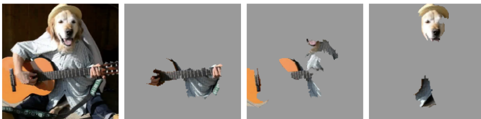
Figure 2.21: Inception’s top-3 predictions (“electric guitar”, “acoustic guitar” and “labrador”, respectively) explained using LIME [SG16]. The highest contributing super-pixels were kept, while the remaining ones were greyed out.
