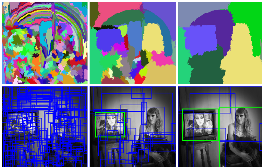
Figure 2.3: Visualisation of how the selective search algorithm progresses [GS13]. The top row contains the segmented regions, while the bottom row contains the corresponding bounding boxes. The algorithm works by joining similar regions together until a stopping condition is reached.
