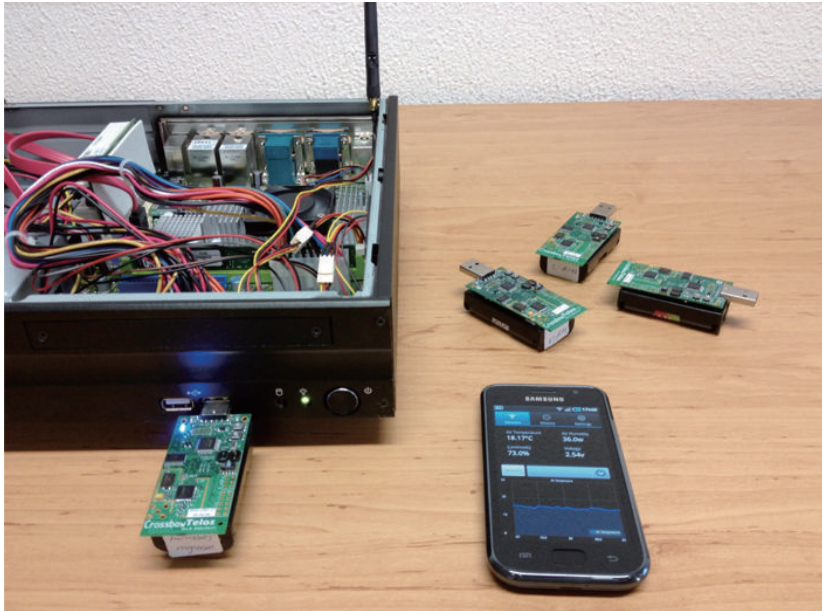
Fig. 9. 6LoWPAN wireless sensor network laboratory testbed.
