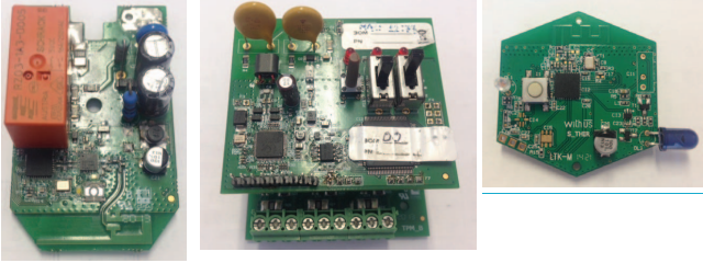
Fig. 2. IEEE 802.15.4 smart plug (left), PLC nodes (center) and IEEE 802.15.4 temperature sensor (right).
