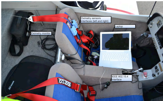
Figure 4. Testbed equipment inside the light aircraft.
