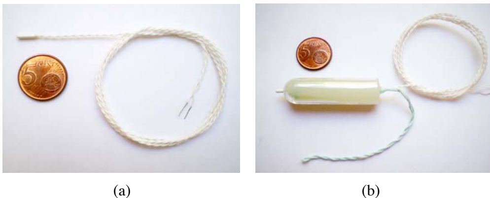
Figure 5. (a) MA100 thermal sensor. (b) MA100 inside enclosure tampon resembles.
