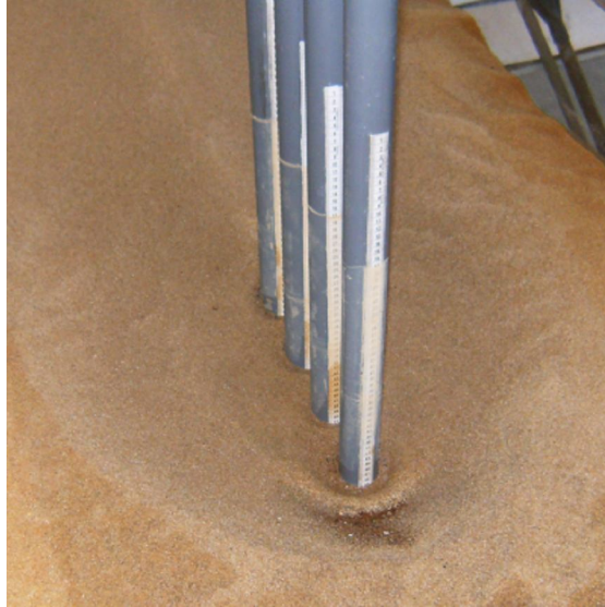
Figure 3.14 – Metric tape glued at each individual pile (FEUP only)
