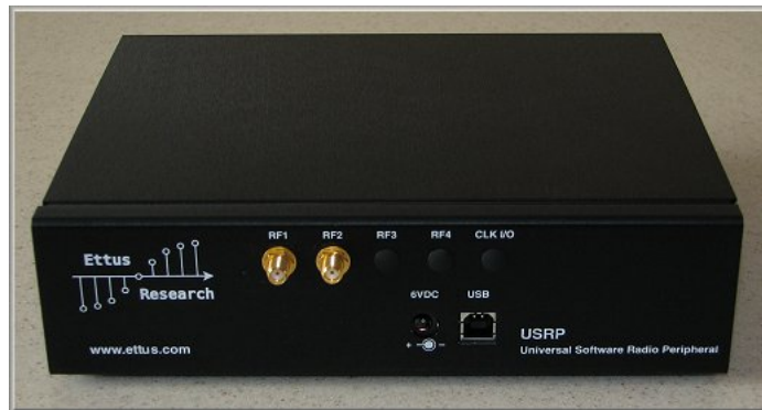
Figure 3.4: Example of a GNU Radio USRP (Universal Software Radio Peripheral) installed in its bulky case.
