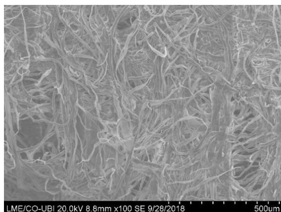
Figure III.49. SEM image of the industrial towel paper sample TW_IND_A.
