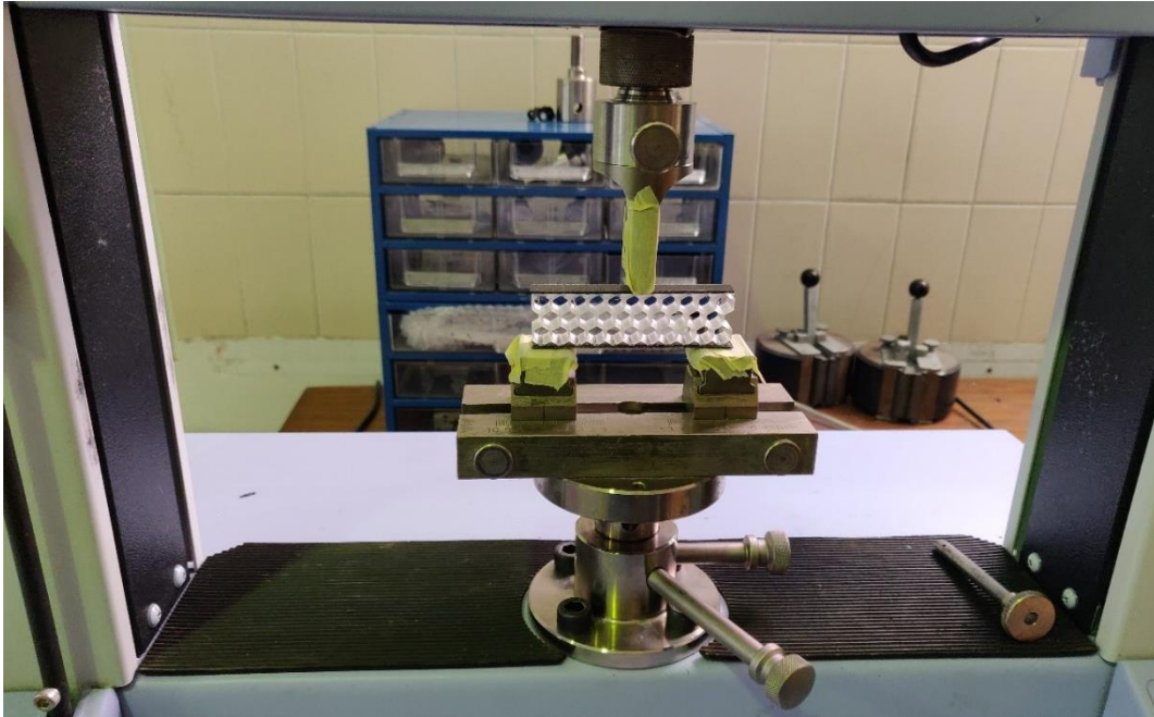
Figure 3.17 – A hexagonal-celled sample ready for the three-point bending testing.
