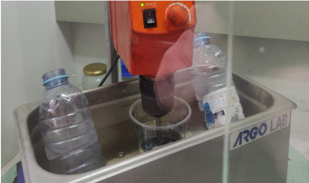
Figure 3.12 – Resin/Carbon nanotube blend undergoing mixing.
