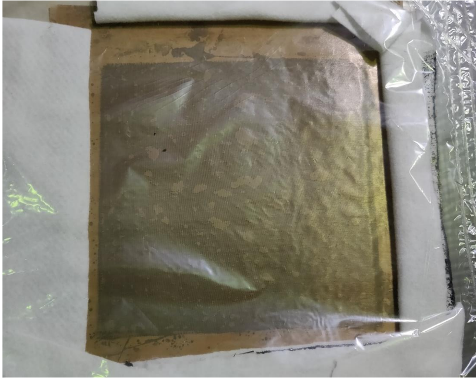
Figure 3.13 – Composite bundle, prior to being inserted into the vacuum bag.
