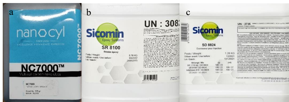
Figure 3.11 – The three components that make up the resin mixture: a, carbon nanotubes; b, resin; c, hardener; reproduced from [30], [31].
