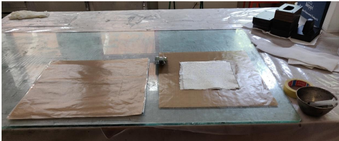
Figure 3.10 – Fibreglass sheets cut into squares and ready for the layering process.
