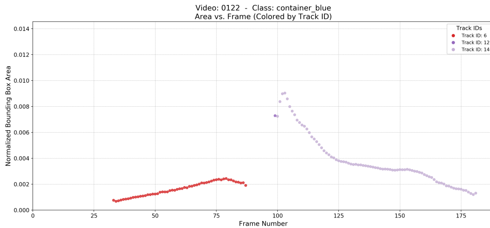
Figure 3.4: Area trajectory showing a track fragment caused by occlusion. The baseline tracker segments this into separate tracks (each track ID is uniquely color-coded to improve distinction).
