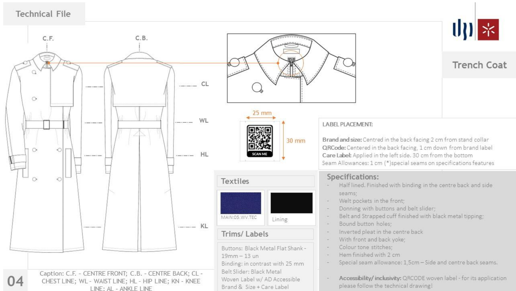
Figure 25. Example of QR Code Woven label application in the garment – Trench Coat.
