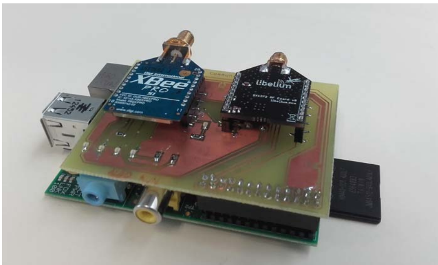
Figure 4.14: Assembled board with both radios plugged into Raspberry Pi.
