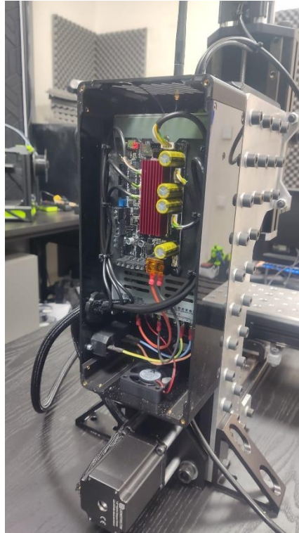
Fig. 81 Electronics enclosure without the cover, allowing the access of the electronics components.
