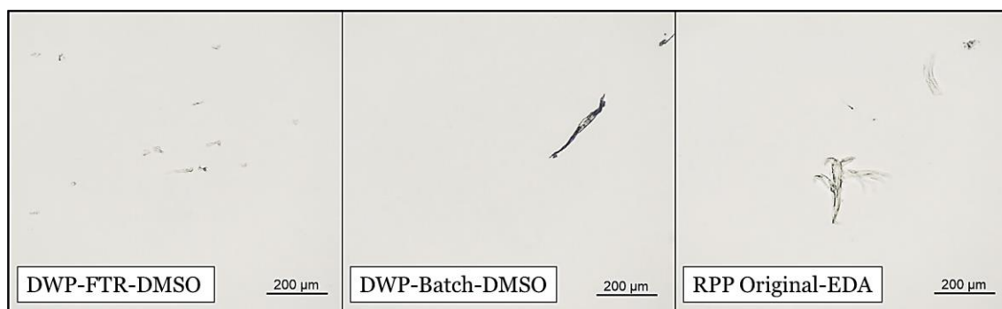
Figure 4.16. Microscopy images (40x) of pre-activated samples for dissolution extension evaluation at 8%LiCl/DMAc solvent system.
