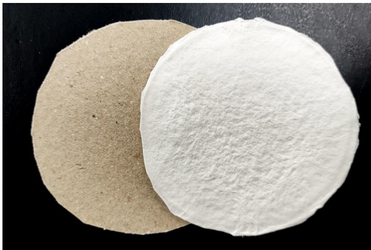
Figure 4.7. Sheets of RPP-Original (left), and RPP-C 3 (right) used for ISO brightness analysis.
