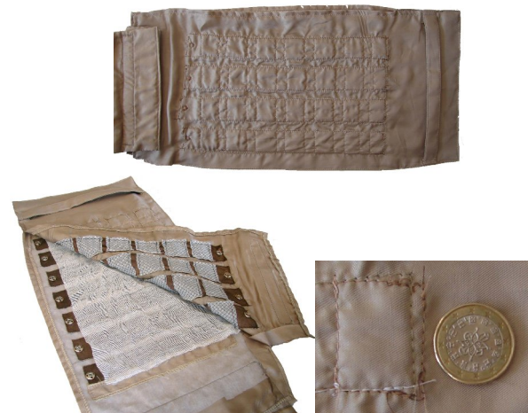
Fig. 4. First Smart-Clothing belt with fabric pressure sensor.
