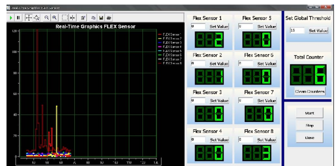
Fig. 10. Print Screen from the software used with the third belt to show the deformation angle in each flex sensor .
