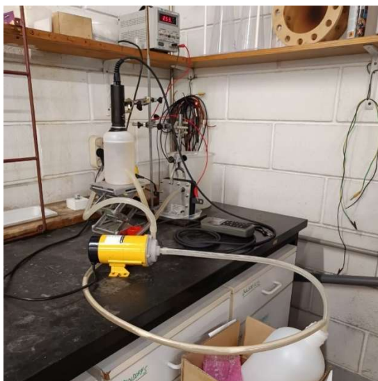
Figure 8. Electrochemical oxidation schematic for MCTW tests.
