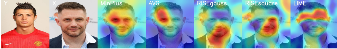
Figure 2.15: Results obtained from [10] on an impostor pair example. Y corresponds to the gallery image, X corresponds to the probe image, MinPlus and AVG are the algorithms proposed by [10] and [4] respectively. RISEgauss, RISEsquare and LIME are adaptations of the methods proposed by [2] and [1].
