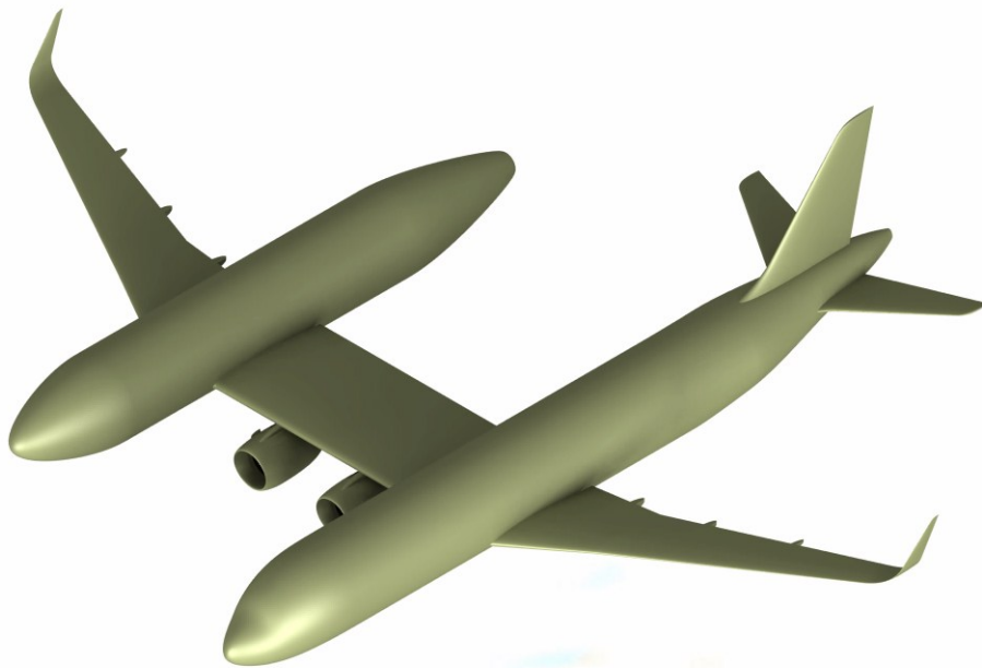
Figure 3.28 - Isometric view of the gondola airliner with winglets, FTFs and A320's tail.
