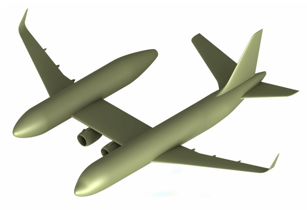
Figure 3.38 - Isometric view of the gondola airliner with winglets, FTFs and a resized tail.
