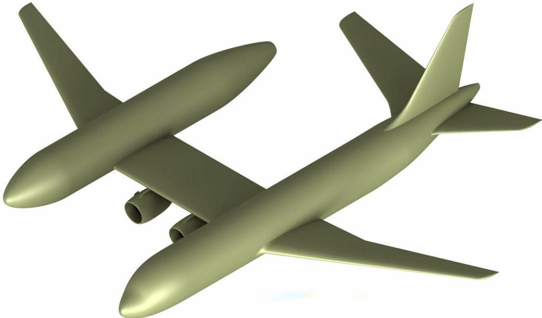
Figure 3.43 - Isometric view of the gondola airliner featuring a resized tail, without winglets and FTFs.
